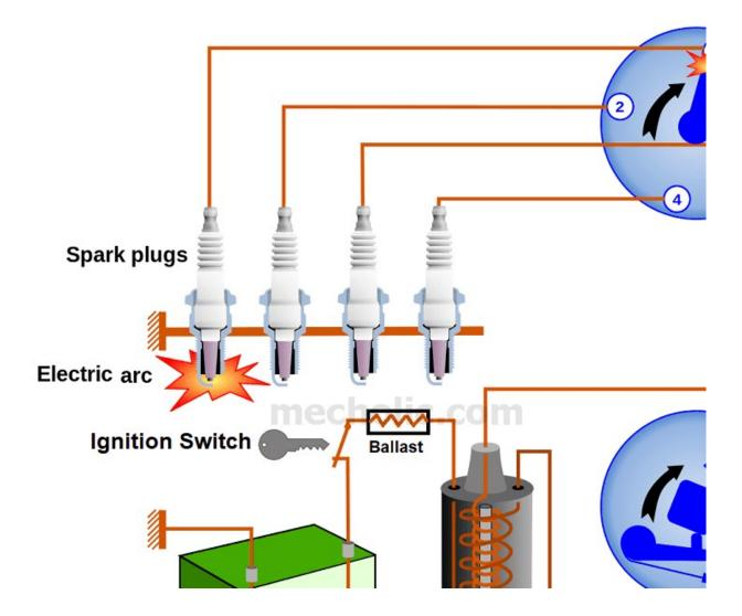
The value of the voltage depends upon the number of turns in each coil. The high voltage, 10,000 to 20,000 volts, then passes to a distributor.
