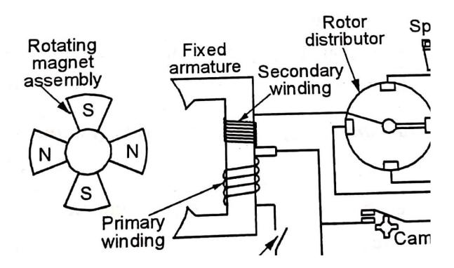
It consists of either rotating magnets in fixed coils or rotating coils in fixed magnets. The current produced by the magneto flows to the induction coil, which works like that of the battery ignition system.
