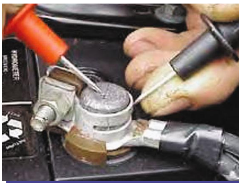
Fig. 4.6 To test the voltage drop of the battery cable connection,
