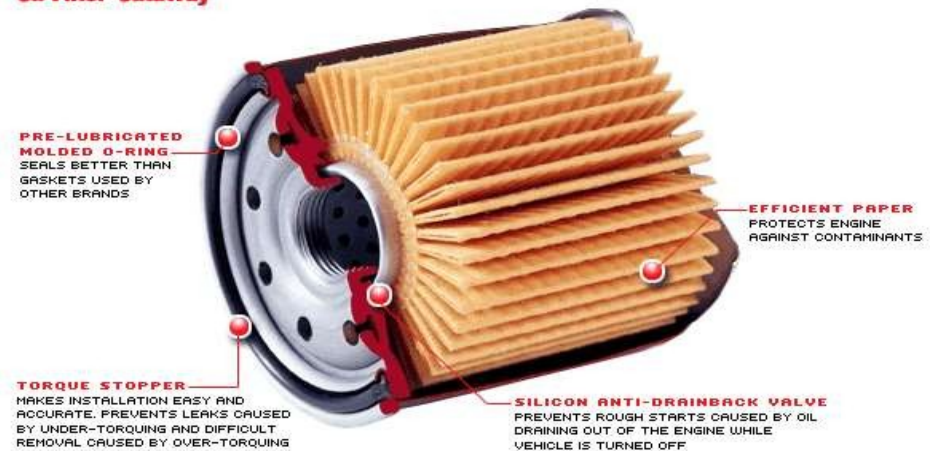
Oil Filter Cutaway
